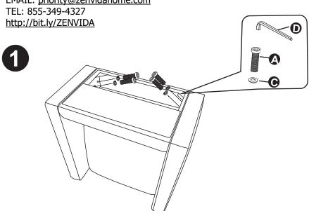
Put the screws in the holes, tight the screws, but not too tight, 90% is ok.
