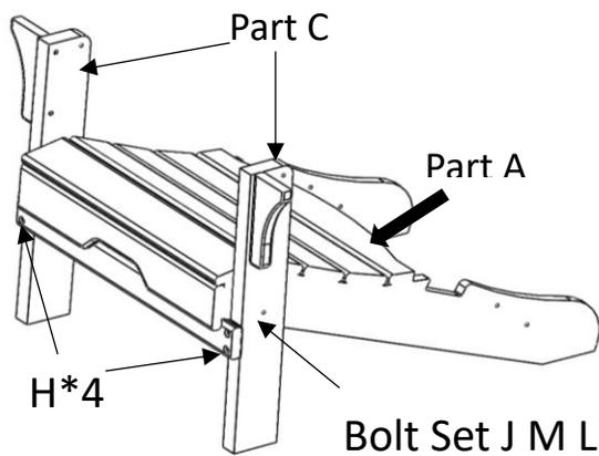
**STEP 2:** Attach the Right and Left Armrests (D) to the Front Legs (C) using 2.6" Bolts (J). Secure with Washer (M) and Nut (L).
