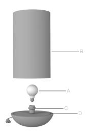
Step 1: Install the light bulb (A) into the lamp holder (C).
