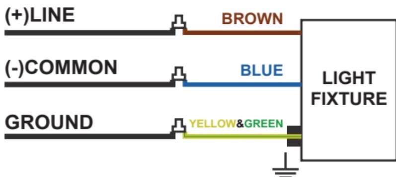
**Step 1:** Connect the bare copper ground wire (yellow and green) from fixture to supply ground.
