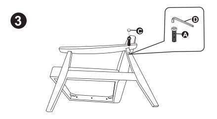
Put the screws in the holes, tight the screws, but not too tight, 90% is ok.
