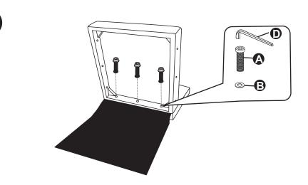
Put the screws in the holes, tight the screws, but not too tight, 90% is ok.
