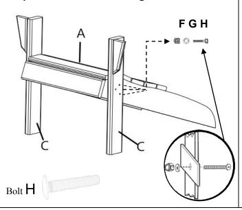
**STEP 2:** Attach both Arm(D) to front legs using carriage bolt 2.55"(H), secure with washer and nuts (G+F) as per diagram, with(M)&(N)
