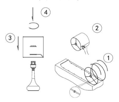
①② Place the two rollers on the lampshade in the same direction as shown in the figure, and press them on the plastic buckle to make them completely coincide, pay attention to the inner installation of the roller protruding part towards the lampshade.
